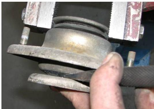
8. Remove the existing rubber bush from the top part of the mount. Remove any paint, rust, burrs or sharp edges from the face of the mount and install the replacement bush 4020 using liberal amounts of grease supplied on contact surfaces (as per diagram C)
