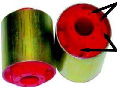
**Stepped pin voids** - These small voids are stepped and only travel through a 1/3 of the way into each side of the bush. This allows for greater rotational articulation and passenger comfort, with no increased Noise, Vibration, Harshness (NVH). This leaves the centre 1/3 to prevent camber & caster movement that the original rubber bushes suffer from and provides better steering feedback to the driver.
