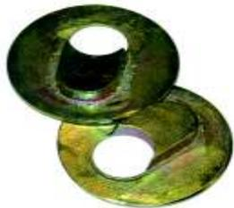
**Nolathane's** rear toe & bump steer correction kit **46268** utilises specially designed locating washers to positively lock the rear toe link. They correct the vehicle's toe/bump steer characteristics by the way the toe link is mounted in relation to the chassis slot. The kit includes 4 x specialty washers which can be used with the original bushes and does not induce N.V.H. (Noise, Vibration or Harshness).
