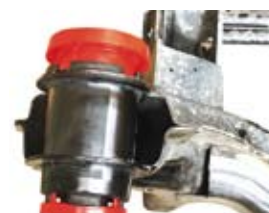
Nolathane kit 49169 being fitted to the original rear cross member bushings
