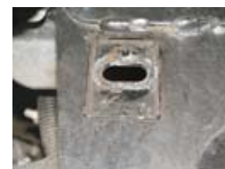
Inner Control Arm Mounting Slots which allows slippage and caster setting changes. Nolathane 45572 kits prevents this movement.
