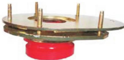
The original strut mount housings are removed and discarded from the vehicle and replaced with the two adjustable strut mount housings provided. The original old rubber mounts and bearings are also removed and replaced with new urethane mounts and OE style bearings.
