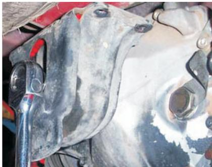
The third mounting point, on the rear of the differential, is a steel housing containing a soft, heavily voided, rubber and steel mount. Over time this mount becomes excessively soft permitting too much movement also leading to axle tramp. The **Nolathane** diff inserts simply press in and are shaped to fill the voids in the original reusable mounts.
