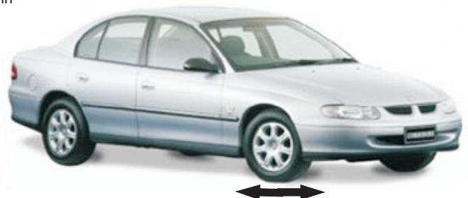
Watch front wheel movement during low speed braking
