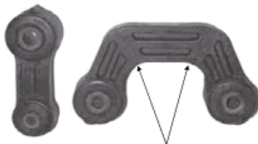
O.E. links & O.E. bushes - check for cracks here.
