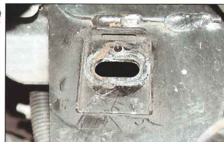
Inner control arm mounting slots which allows slippage and caster setting changes. Nolathane 45572 kits prevent this movement.
