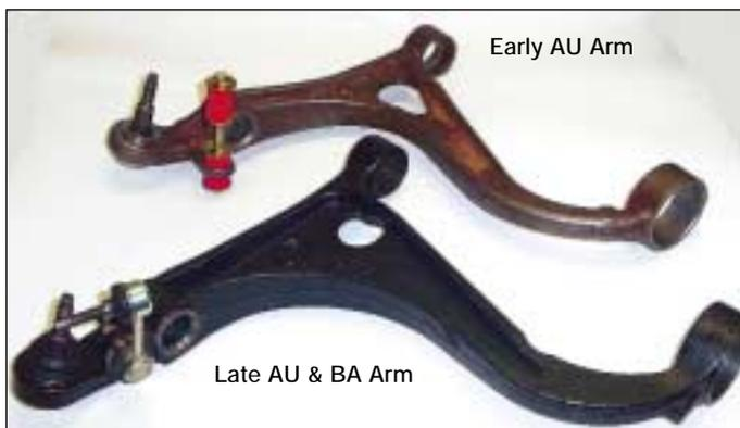
improved retention of alignment setting with less movement under braking and cornering. An improved brake pedal feel is also evident along with reduced tyre wear.
