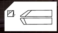
It is best to bore Nolathane solid rod and mount it on a mandrel for the best turning results - the same applies when modifying moulded bushes. Having the tool approximately 1mm below centre height removes material a lot easier, No coolant is necessary if these procedures are followed.
