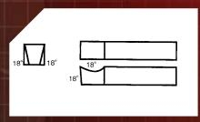
In some applications you will want to machine a groove or recess into the outside dimension of the part you are making. This is best carried out by plunging a shaped tool into the part. Head speed and surface feed should be the same as for turning procedures.
