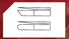
Either a parting tool or old power hacksaw blade can be used. For best results sharpen your tool to a razor edge point - a bull nose or flat nose with slight backrake can be used.
