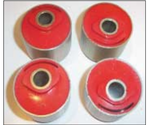
Shows voiding in offset castor bushes
