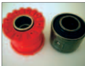
Nolathane voided design compared to Subaru hydraulic front lower control arm inner rear bush.
