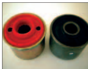
Nolathane voided design compared to Mitsubishi hydraulic front lower control arm inner rear bush.
