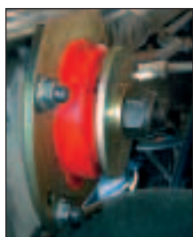
Nolathane strut rod bush fitted to Commodore.
