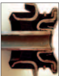
Cut-away of failed Commodore strut rod bush. Note voided area (hydraulic fluid reservoir) around centre of bush.
